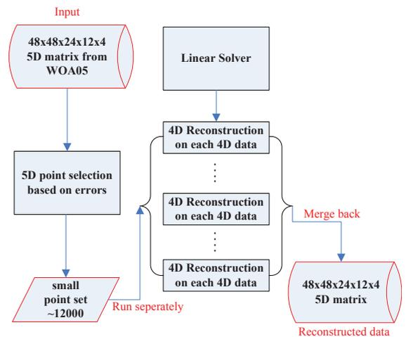
Figure 2: 5D-ODETLAP Algorithm Outline
